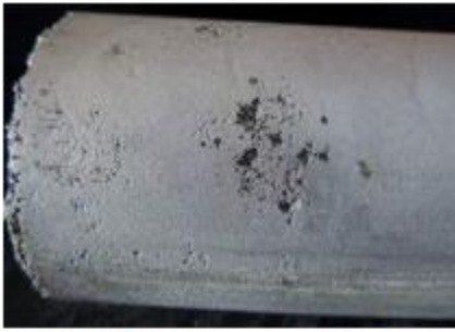
Figure 17.17 Pitting of a 316L stainless steel pipe surface by a phosphate solution. (Photograph courtesy of Rick Adler/Adler Engineering LLC of Wyoming USA)
