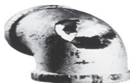
Figure 17.20 Impingement failure of an elbow that was part of a steam condensate line. (Photograph courtesy of Mars G. Fontana. From M. G. Fontana, Corrosion Engineering , 3rd edition. Copyright © 1986 by McGraw-Hill Book Company. Reproduced with permission.)
