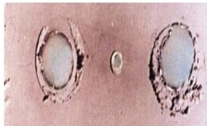
Figure 17.15 On this plate, which was immersed in seawater, crevice corrosion has occurred at the regions that were covered by washers. (Photograph courtesy of LaQue Center for Corrosion Technology, Inc.)
